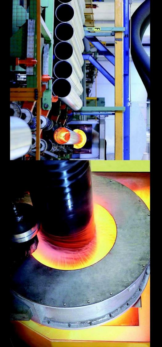
Rivit's heat treatment department has both induction and batch type furnaces which are calibrated in accordance with ASTM A 991 and API 5L for annealing and stabilising of all materials.
