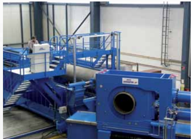
The new electric induction machine Schäfer SRBMI 1400.
