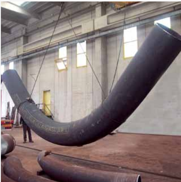
Large radius bend pipe manufactured by OMP-Mongiardino - Tectubi Raccordi Bending Division.
